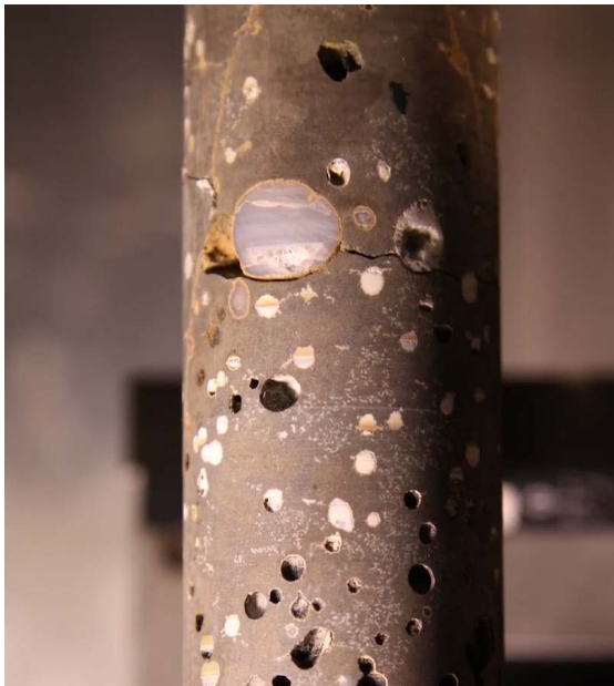
Figure 7. Core from a well near Wallula in southeastern Washington showing calcium carbonate nodules (light color) resulting from carbon mineralization. The core sample was taken from a well two years after 977 MT CO 2 were injected into the Grande Ronde basalt at a depth of nearly one kilometer, or 3,281 feet, during the summer of 2013. The light areas show portions of the rock where calcium carbonate minerals have replaced the original basaltic minerals. 96
