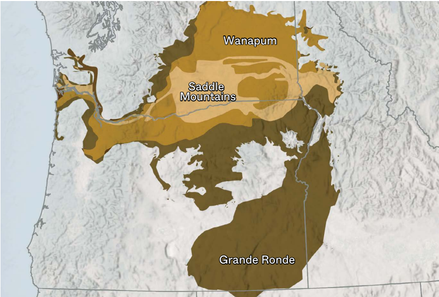
Fig. 2. Generalized geologic map of the CRBG showing surface extents of three major basalt formations and their layered stratigraphy. Surface extents are visualized axonometrically.
