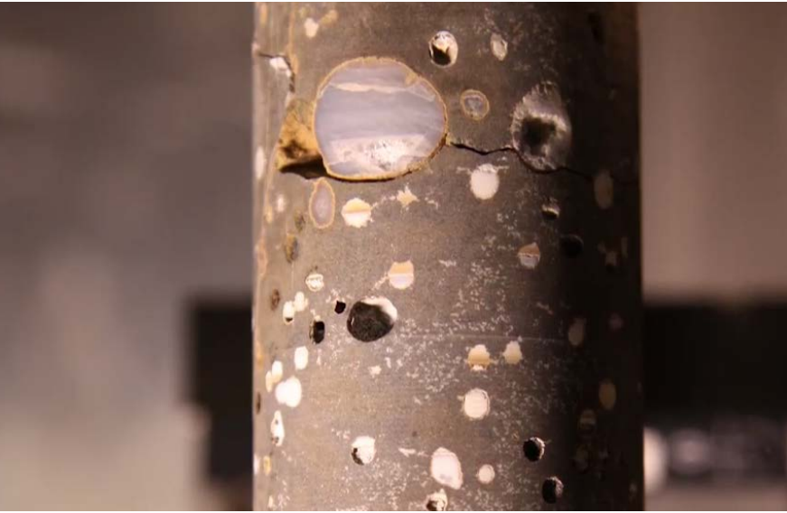
Fig. 4. Drill core showing calcium carbonate nodules (light color) resulting from carbon mineralization. Pacific Northwest National Laboratory .
