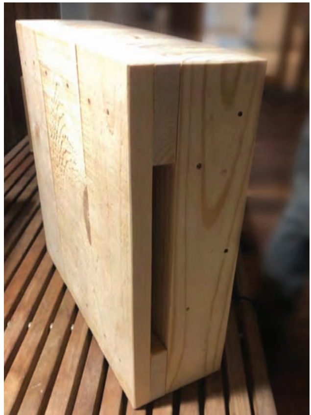
△ Figure 6. Panel prototype with yellow pine and Lignoloc® nails for Guilford Demonstration Building.
